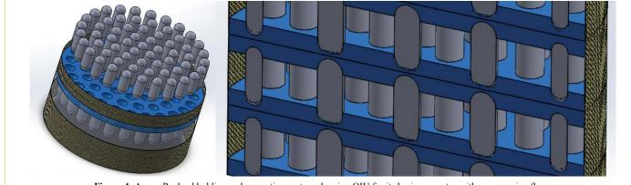
Figure 4: A new Payload holding and separation system showing OIU for its basic geometry with compression floor.
