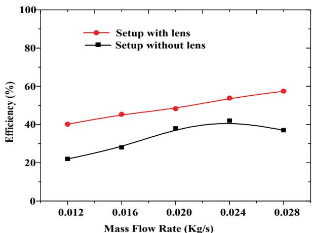
Figure 13: Comparison curve of Mass flow rate vs. overall efficiency.
