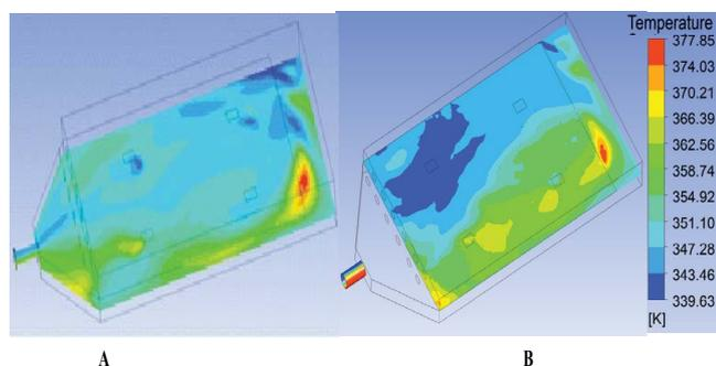
Figure 7: Temperature distribution on the surface plane below and above the collector plate of double pass solar air heater.
