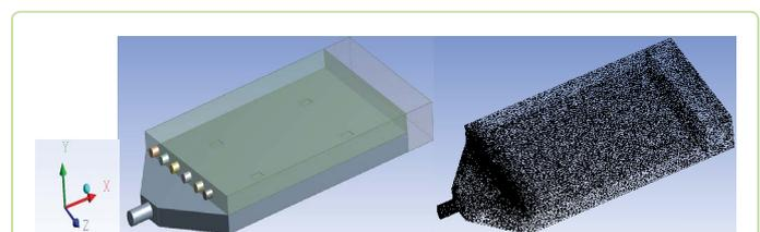
Figure 5: Double pass solar air Heater with adopted mess.
