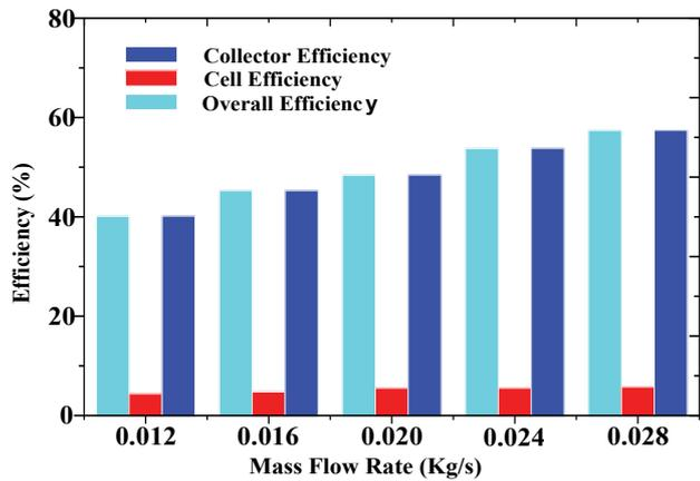
Figure 10: Effect of cell efficiency on overall efficiency.
