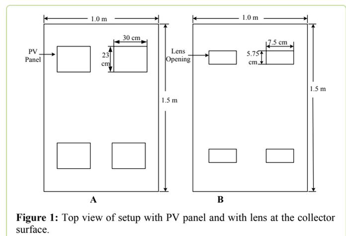
Figure 1: Top view of setup with PV panel and with lens at the collector surface.
