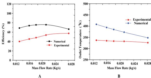
Figure 12: Variation of efficiency and outlet temperature due to mass flow rate.
