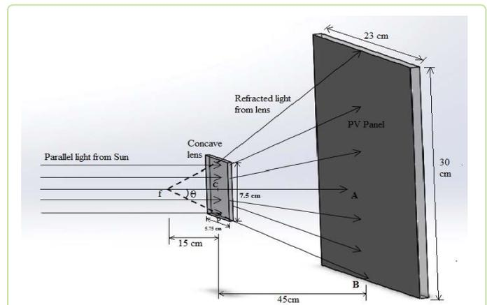
Figure 2: Ray diagram to measure distance between lens and solar panel.
