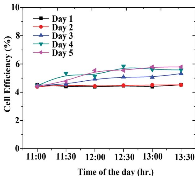
Figure 9: Time of the day vs. cell efficiency curve.
