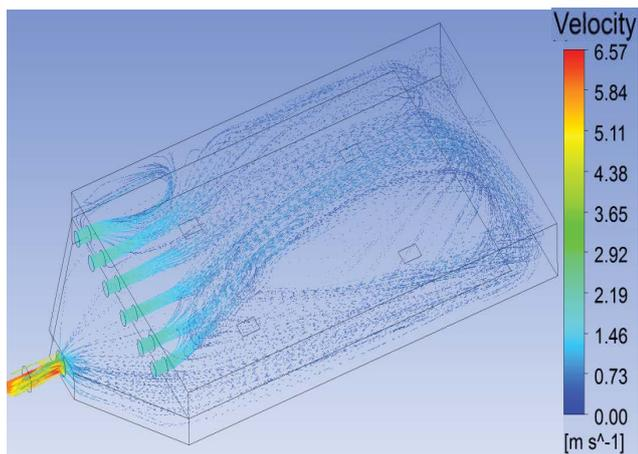
Figure 6: Velocity vector of flowing fluid within the double pass solar air heater.
