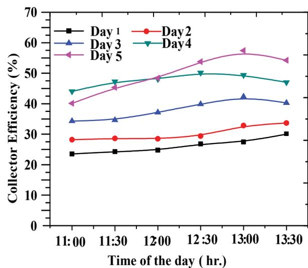
Figure 8: Time of the day vs. collector efficiency curve.
