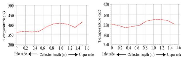
Figure 11: Temperature Distribution above the absorber plate for lower and higher mass flow rate.
