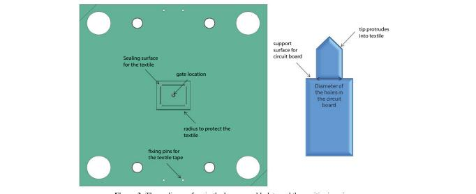
Figure 3: The sealing surface in the lower mould plate and the positioning pins.
