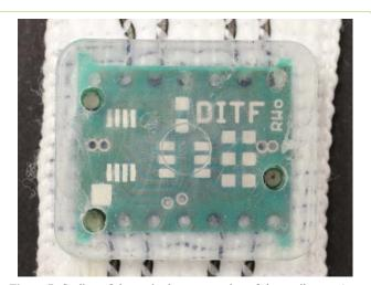
**Figure 7:** Sealing of the cavity by compression of the textile tape (test series 4 from the full factorial test plan).
