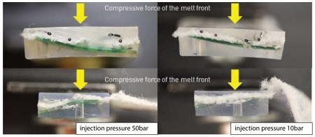
Figure 4: Deformation of the circuit board caused by variation of the injection pressure.
