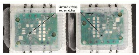
Figure 5: Surfaces of test series 1 (left) and test series 2 (right) of the full factorial test plan.
