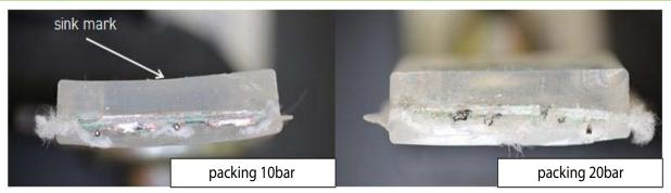
Figure 8: Reduction of the sink mark caused by a higher packing pressure.
