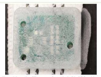
**Figure 6:** Incomplete filling pattern of test series 3 of the full factorial test plan.
