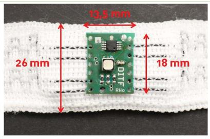
Figure 1: Picture of the inserts (textile tape and circuit board) and dimensional data.
