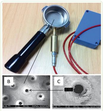
Figure 6: (a) Portafilter and coffee basket. (b) Coffee Basket holes (c) 336.6  $\mu$ m Extraction hole size.
